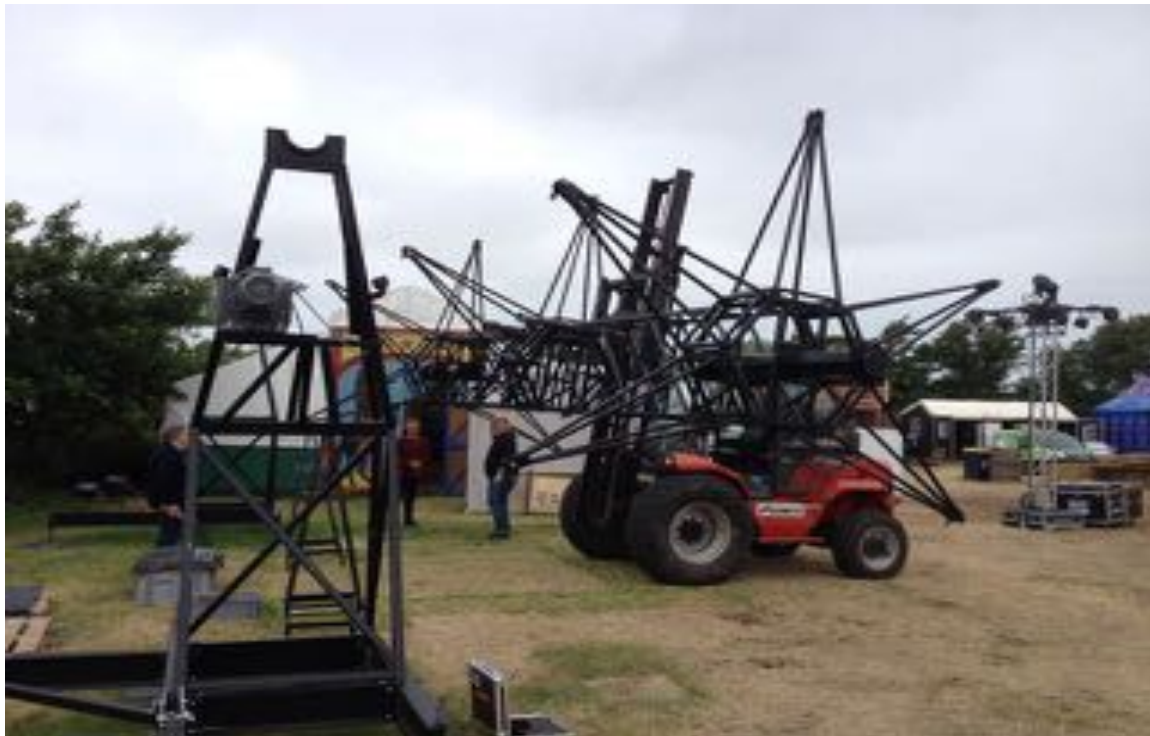
Setting up with Manitou M30-4 all-terrain forklift:
